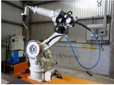
Robotic Welding Machine
